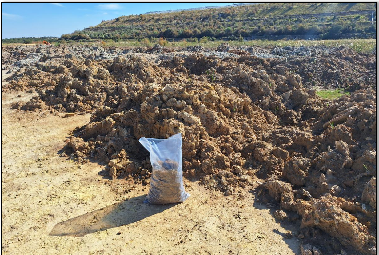
Plate 23. Sampling of soil stockpiled across the south-western portion of the site between TP1 and TP3.
