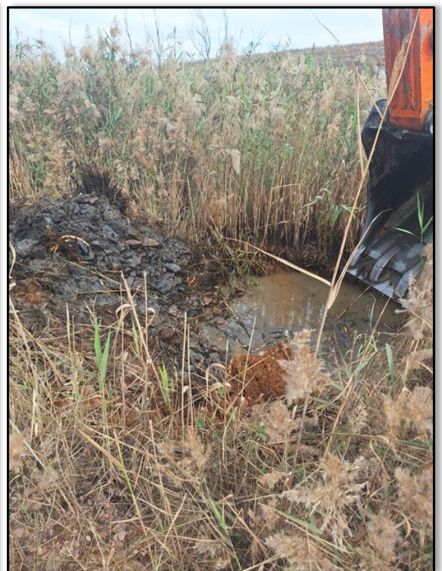
Plate 49. Saturated test pit at TP25.
