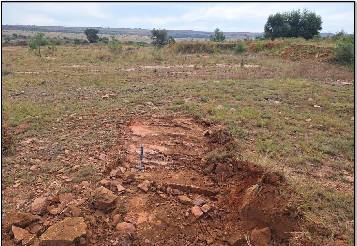
Plate 7. Shallow bedrock with outcrops at test pit TP23.
